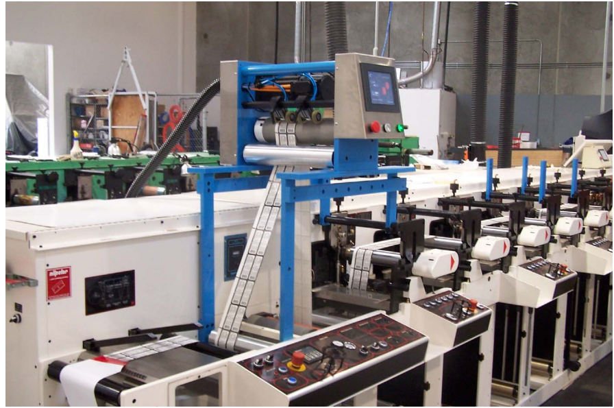
A Servo3000 Digital Re-register System™ is positioned above the infeed station of a web press. Note the alternate mounting location for the Servo3000 a few stations to the right. Using the Xycom HMI/PLC, an operator can quickly re-configure the re-register unit after moving it to a different station or press.
