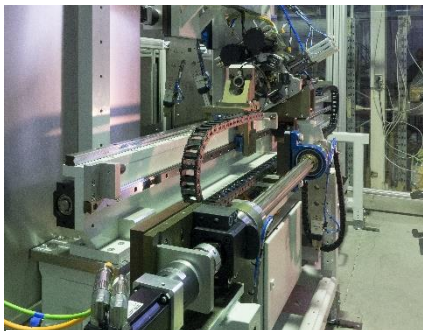
Tilting axis for retrieving blanks from the drum magazine, driven by the Kollmorgen AKM servo motor.
