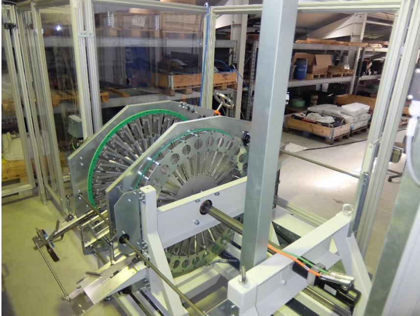
Drum magazine serves as a buffer for blanks, driven by the Kollmorgen AKM servo motor
