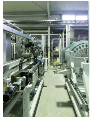
View of the equipment, with drum magazine, tilting axis and cutting head.
