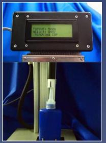
**Built-In Validation** – Because of the built-in force, torque, speed and stroke feedback on each actuator, the presence of a cap and proper on- and off-torquing are all performed and validated using the same SMAC actuator. All this is validated on the dial so no additional downstream inspection stations are needed.
